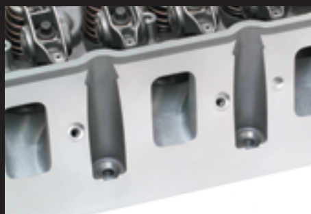
LS7 2006 7.0L V-8 (LS7) Cylinder Head - Intake Ports for Corvette Z06.
