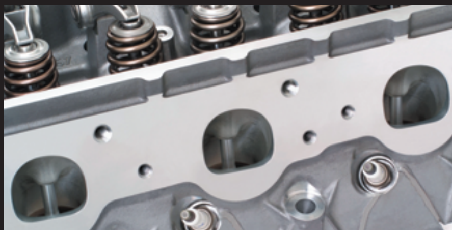
LS7 2006 7.0L V-8 (LS7) Cylinder Head - Exhaust Ports for Corvette Z06.
